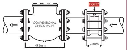
DUAL FLAP WAFER CHECK VALVE
