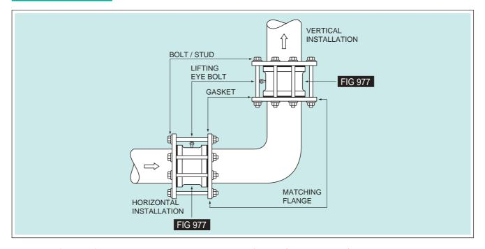
AFA dual flap wafer check valves need one sets of bolts (studs & nuts) to install it. These check valves installed in horizontal position must be installed with hinge pin in the vertical position to ensure proper operation. AFA check valves larger than 6" (DN150) are fitted with lifting eye bolts to provide easier handling and site safety.
