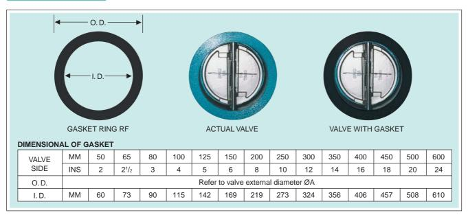
Use the correct dimension of gasket especially I.D. is important. The correct dimension of gasket (O.D. = valve external diameter ØA and I.D. = valve internal diameter ØB) provide a perfect opening of disc and prevents leakage as well.
